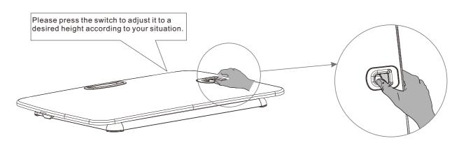
When lifting the workstation, press the switch by your thumb and up the table with holding both sides of table edges, then it will get next height ,locked asthmatically when you hearing the voice. When lowering the workstation, press the switch by your thumb and the loading will let it lower from current height, locked it automatically when hearing the voice.
